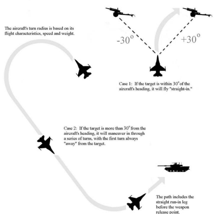
Figure 390: Aircraft flight paths as set by the Al based on the relative target location and final heading required.
