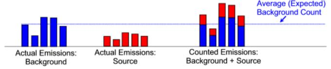
Figure 85: Example of how actual radiation emissions and counts will vary randomly around an average value. The differences between the individual counts are relatively exaggerated for illustration purposes, and in most practical cases, the counts from the outside source (red) will be much lower than the background counts (blue), making detection much more difficult.
