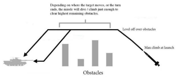
Figure 352: Powered In-flight units follow simple flight paths. If the in-flight munition is guided, the flight path is periodically adjusted to account for target movement.
