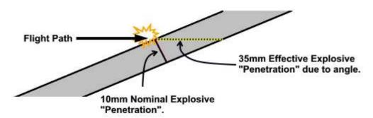
Figure 359: Effective vs. Nominal Penetration for an explosive charge.
