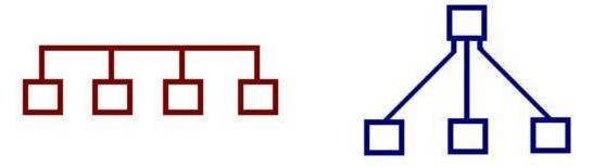
Figure 307: Network types. The red (on the left) is a distributed network, the blue (right) centralized.
