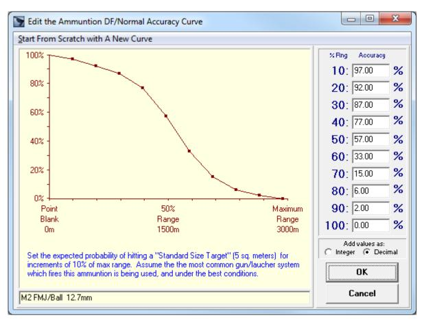
Figure 410: The Ammunition Accuracy Curve Form. This form is used to set the base (i.e., "firing range") accuracy of each type of ammunition. Accuracy is set as the average/expected probability of hitting a "standard size" target (5 sq. meters) over the ammunition's maximum range (in 10% range intervals).
