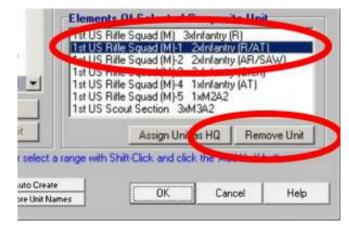
Figure 302: Select a subunit to remove from the Elements in Composite Unit Box then click the [Remove Unit] button.
