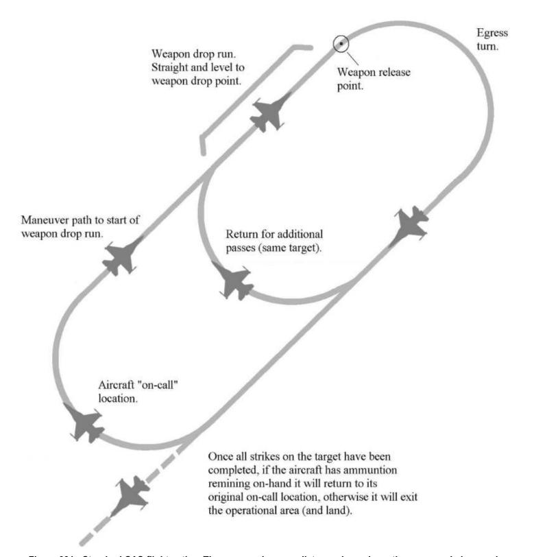
Figure 391: Standard CAS flight paths. The weapon drop run distance depends on the weapons being used.
