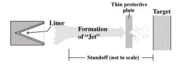
Common countermeasure - thin protective plates cause premature detonation of the warhead outside the optimal standoff.
