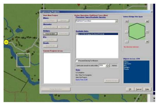
Figure 237: Placing a narrow span bridge in the selected location (white square). The West and Southwest directional buttons are disabled; the bridge is not long enough to span the hexside (river) in those directions.
