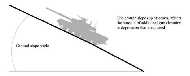
Figure 353: Firing angle considerations for non-powered ballistic projectiles.
